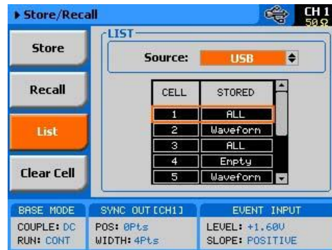
Figure 3-93, Stored Memory Cells Listed
